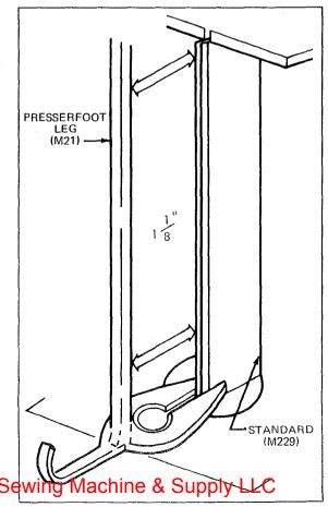
If the Presserfoot Leg is too far in at the bottom, the "Flexi-Bands" will sharpen a wider bevel on the lower portion of the blade. This condition can be corrected by pulling the Presserfoot Leg out slightly and squeezing the Presserfoot Toes together with pliers. This will cause the Presserfoot Leg to set further out at the bottom.
